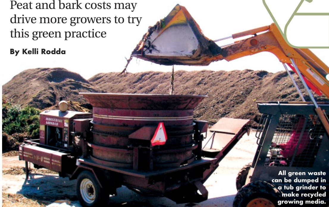
All green waste can be dumped in a tub grinder to make recycled growing media.
